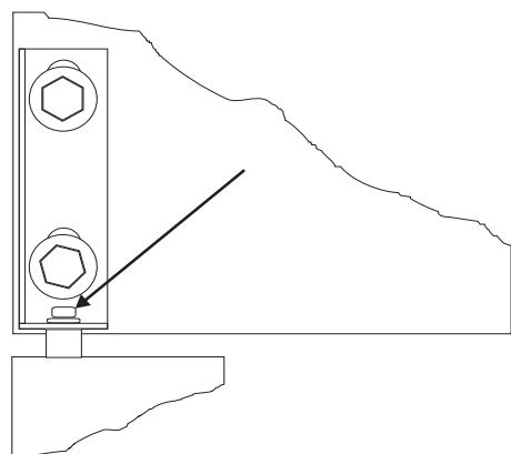
Close and fasten the top with screws as in fig. 1.7.
