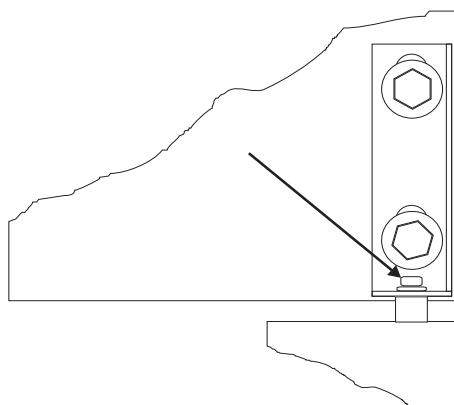
The door is placed horizontally and the door spring and bottom bush are reversed as in fig. 1.4.
