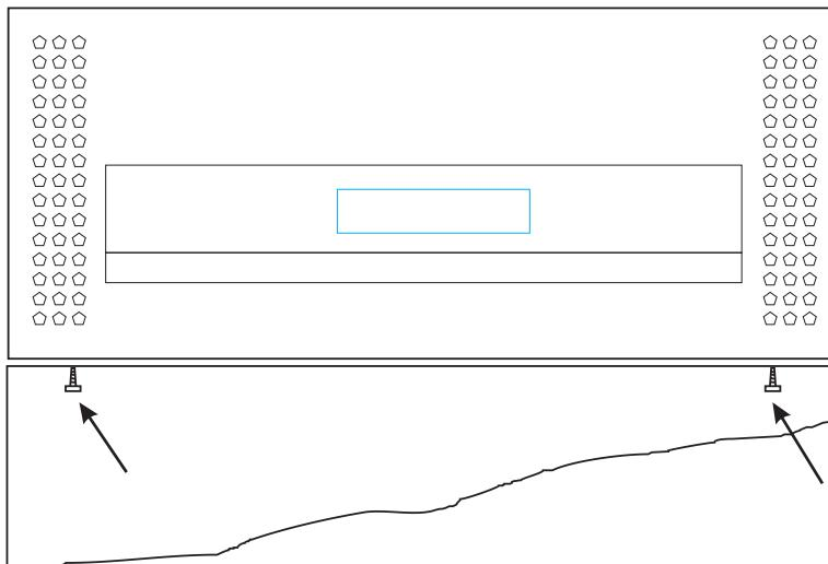
Remove lock screw in door spring as shown in fig. 1.3. Loosen the hinge and remove the door.
