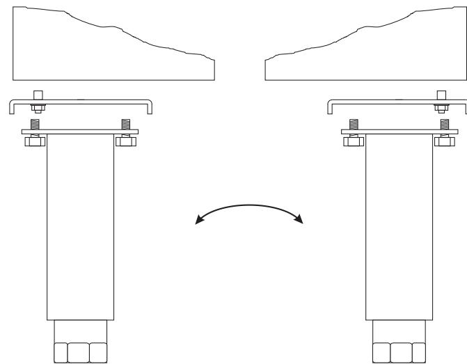
Loosen the top hinge in the new hinge side and replace the door on the bottom hinge. The hinge is pressed downwards on the door spring and is fastened. Put in the lock screw as in fig. 1.6
