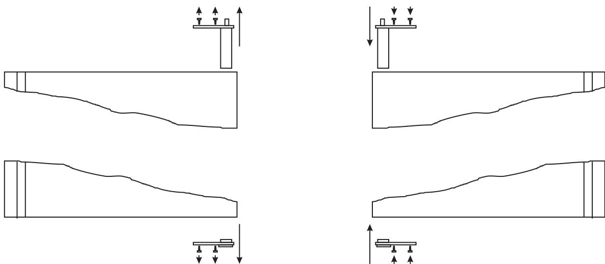
The bottom hinge is reversed by demounting the front legs/wheels and mount them in the other side of the cabinet as in fig. 1.5
