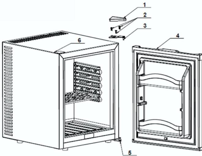
1.Hinge Cover 2.M5X12 Screw 3.Top hinge
